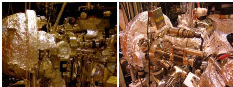
High-efficient spin detection (100 times better than the Mott detector)
