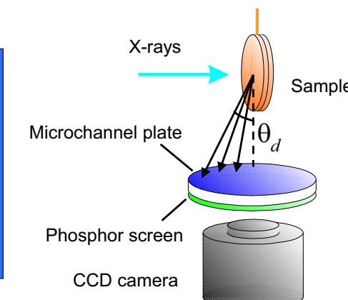
Electron yield XAS measurements at different detection angles
