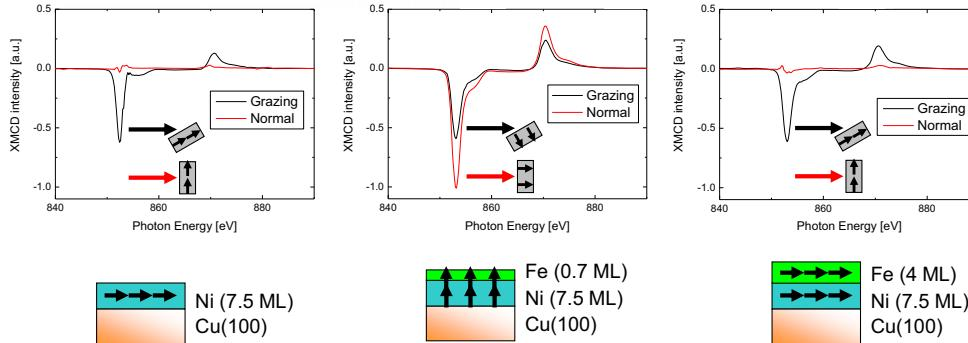
XMCD reflects magnetic component which is parallel to X-ray beam.
