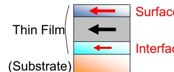
Surface and interface show different magnetism from inner layers
