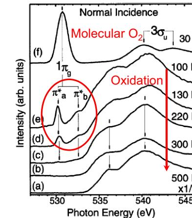
Existence of molecular oxygen in the initial stage of Si oxidation
