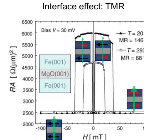
Fig. 3. Magnetoresistance curves for Fe(001)/MgO(001)(20 Å)/Fe(001) MTJ at  $T = 293$  K and 20 K. The MR ratios were 88% and 146%, respectively.
